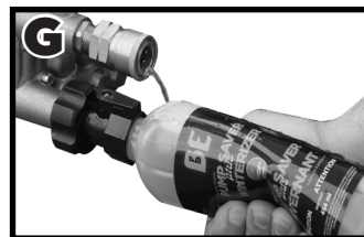
G EVERY 10 PULLS, SQUEEZE BOTTLE TO FORCE FLUID THROUGH PUMP. REPEAT UNTIL FLUID COMES OUT OF OUTLET.
